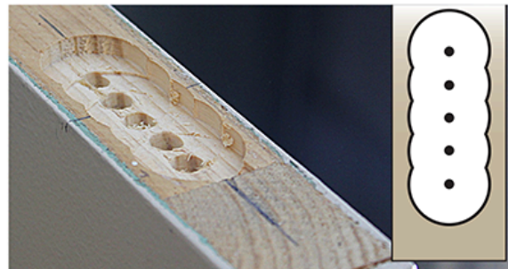
4. Now Bore 2 x more 25mm ( 1'' ) holes into remaining pilot holes ④, ⑤ to remove small side protrusions .
