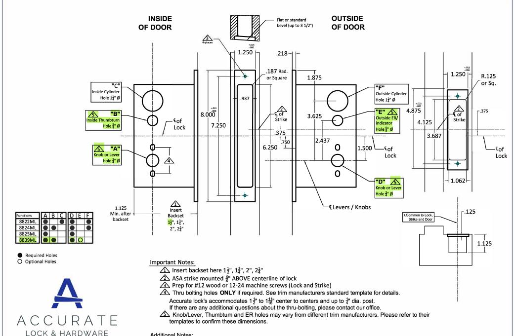
Standard 8800ML Magnetic Lever x Lever or Knob x Knob Template - All Backsets
