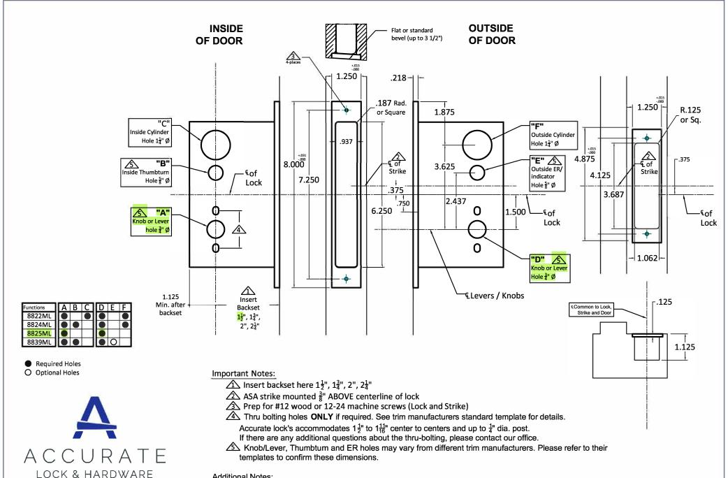
Standard 8800ML Magnetic Lever x Lever or Knob x Knob Template - All Backsets
